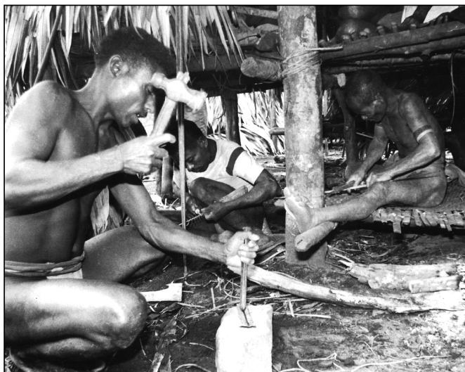
Figure 11. Men making arrow points: front left, cutting out a blank using a hammer and chisel; center, filing a ginilat ; right, shaping a bugwan shaft with a hunting knife. The fire for heating iron is to the front right. Nandukan, Cagayan.
